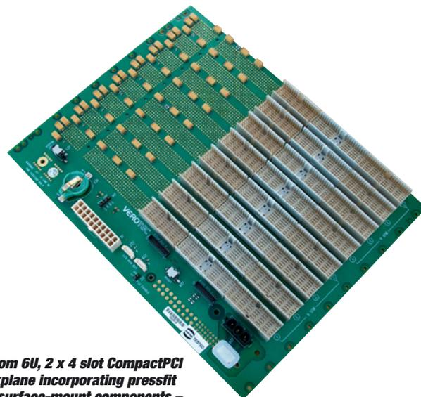
**Custom 6U, 2 x 4 slot CompactPCI backplane incorporating pressfit and surface-mount components – simulation application**
