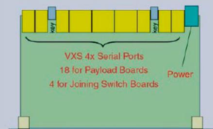
Figure 2. VXS Switch Card
