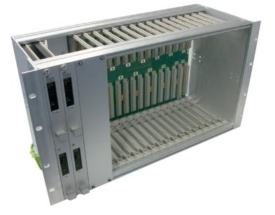
Integrated 6U x 84HP x 180mm KM6-HD IEC subrack , wired with VMEbus backplane & custom H15 power supplies - simulation application.
