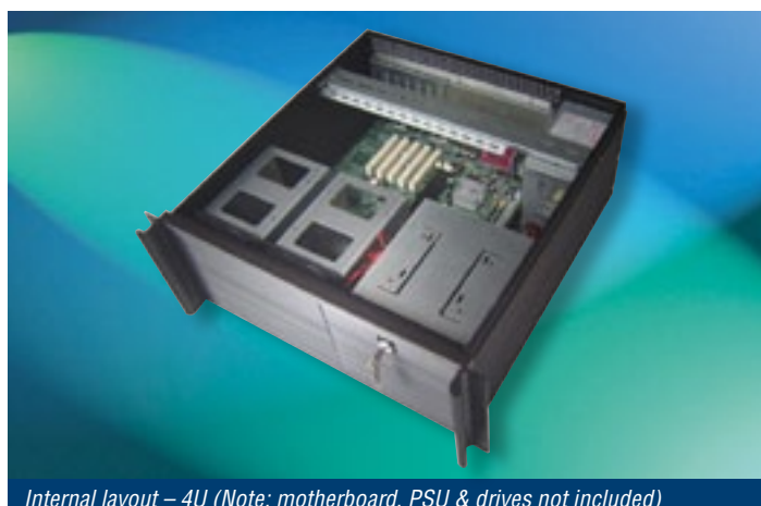
Internal layout – 4U (Note: motherboard, PSU & drives not included)
