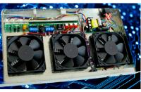
whereas filtered types incorporate 25mm fans, giving room for a removable, washable filter to reduce dust build up. Airflow is up to 120cfm per fan, depending upon the option chosen.
